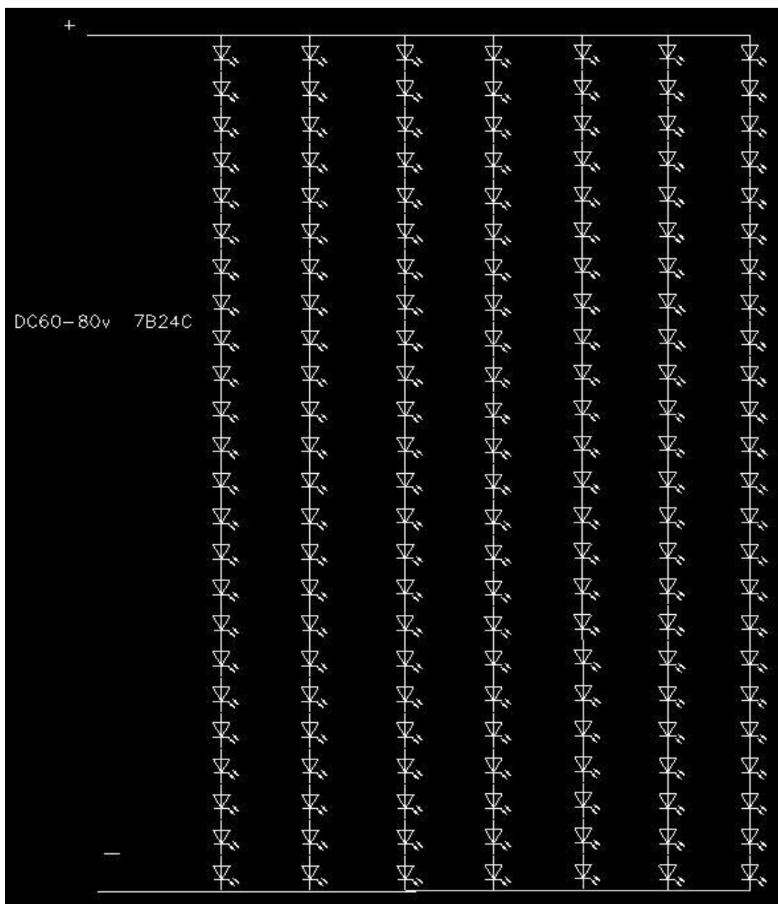
Illustration 8 - Schematic Diagram of LED Module for model SWT81824A2120
